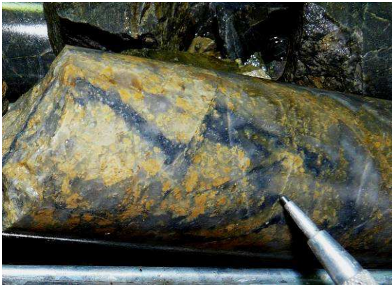
Photo 1: Flaky molybdenite (blue grey) crystals in quartz stockwork vein - 383m DUNDD005.
