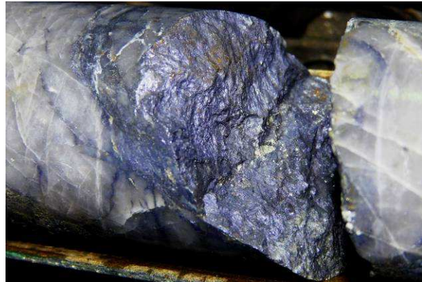
Photo 2: Thick molybdenite vein within quartz stockwork - 512m DUNDD005
