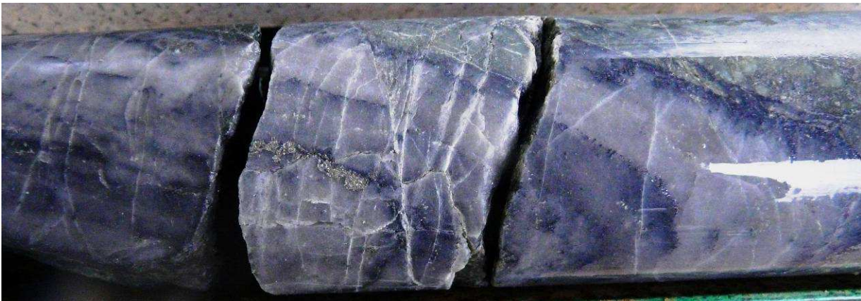
Photo 3: Multiple layered molybdenite and quartz vein - 485m DUNDD005
