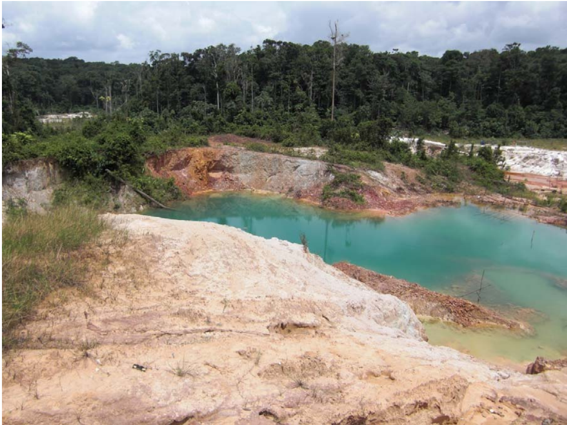
Figure 3. Smart's Pit located approximately 4.5 km along strike from the Hicks Prospect. The Hicks shear zone, can be observed as the brownish yellow (limonite stained) vertical zone in the far left wall of the pit.
