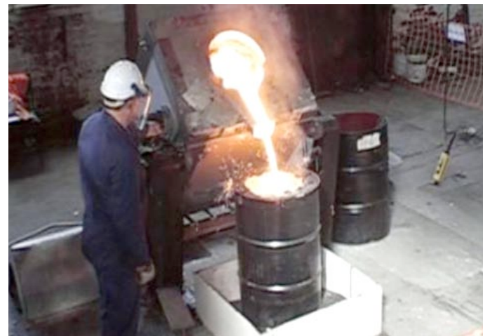
Pouring iron at the Matmor test plant
