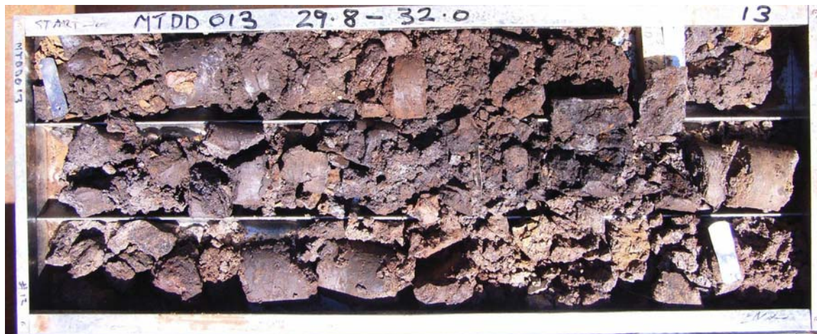
Figure 3a: Hole MTDD013 - 29.8 to 32m, dark cobalt-nickel bearing manganese oxides in broken strongly oxidised ultramafic rock.
