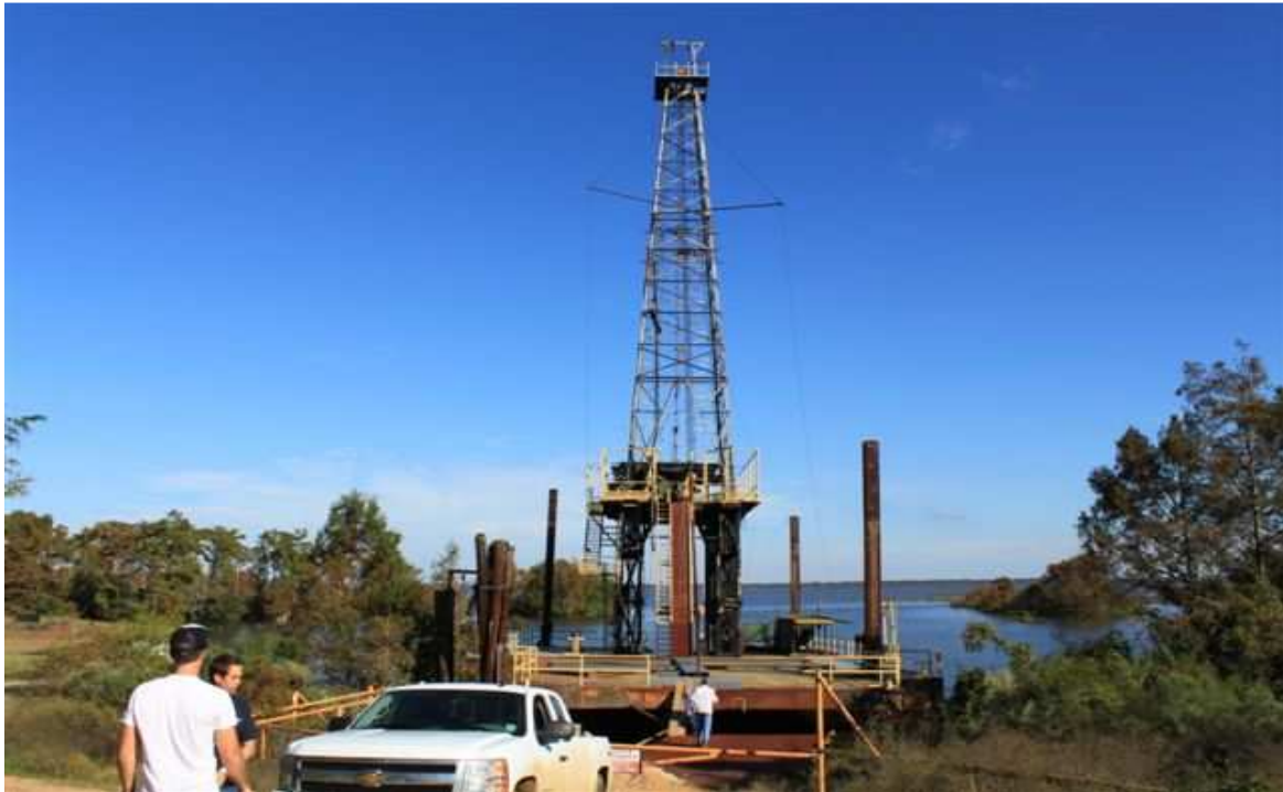
The barge rig used to drill wells on the Lake
