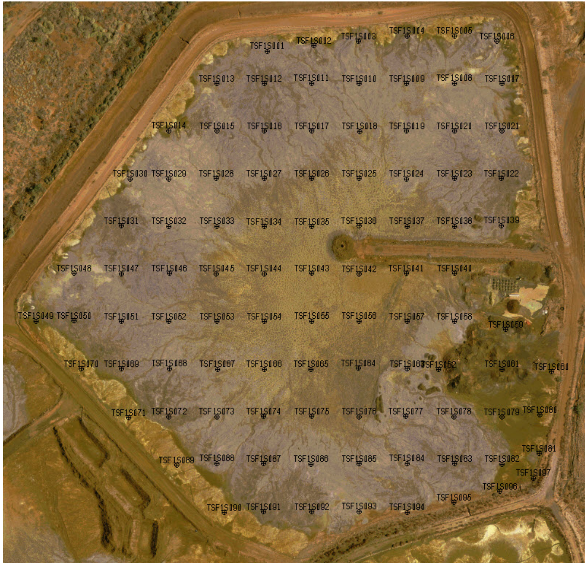
Figure 2: Plan view of drill-hole collars for the drill-out of the TSF1.
