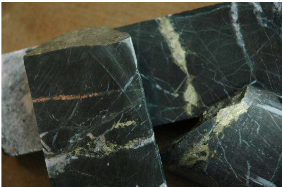
Hole BTDD004- Chalcopyrite and carbonate veining @ 94m.
