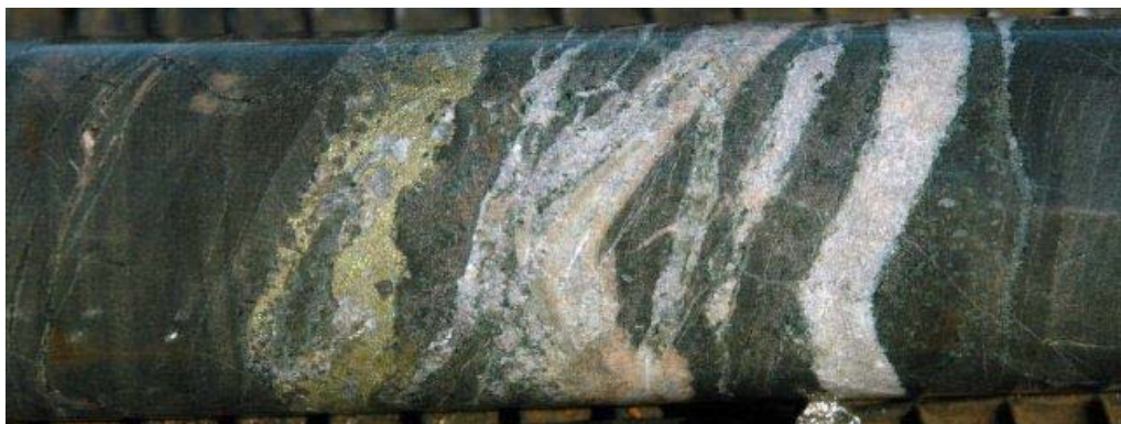
Hole BTDD001- Chalcopyrite Carbonate veins in fresh siltstone @ 68m.
