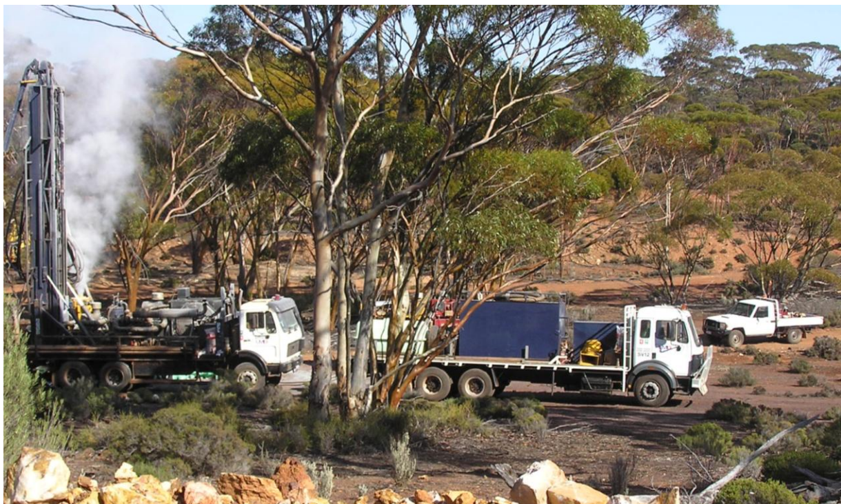
Figure 3: Drilling of the 120m vertical hole up-dip from AEM target intersecting sulphides
