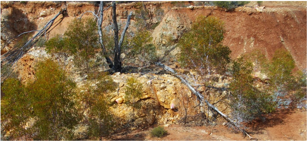
Figure 4: The quartz lode is the white / yellow outcrop in the centre of the 6m deep open cut pit
