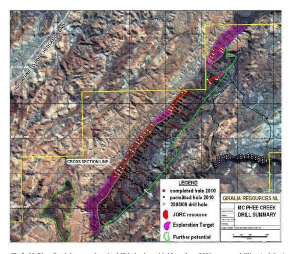
Fig.2; McPhee Creek iron ore deposit, drill hole plan with May –June 2010 resource drilling (red dots)
