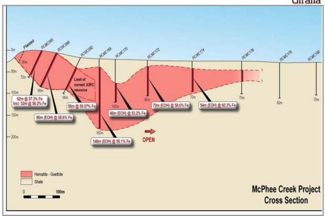
Fig.1; Cross Section McPhee Creek main range deposit (location of section shown on fig.2).
