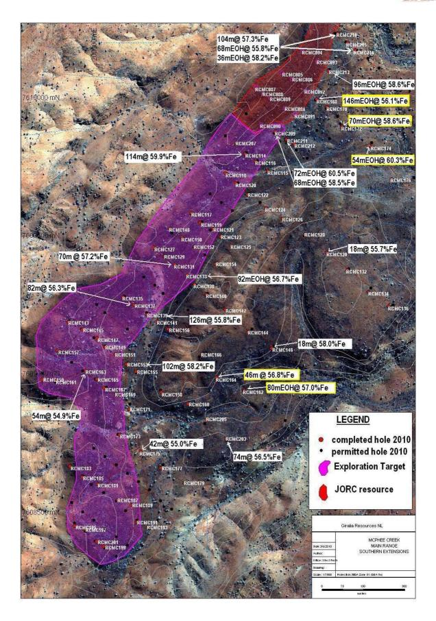
Fig 4; Detailed hole location plan of the southern end of the McPhee Creek main range, showing significant results for holes south and east of the resource. New intersections the subject of this release are highlighted in yellow.
