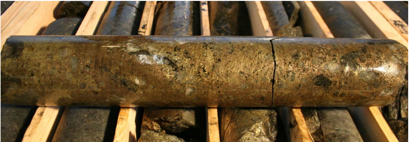
Photograph 1. High grade copper mineralisation from 70.4 to 70.8 m in Hole 12-09 containing chalcopyrite-pyrite-pyrrhotite. This mineralisation makes up part of a 6.35 m intersection (68.80 to 75.15 m) containing 2.38 % copper and 2.85 g/t gold.
