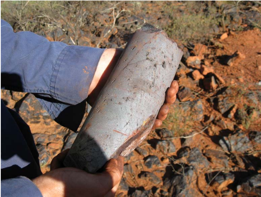
Figure 1: PQ diamond drill core high grade hematite from the John William Douth deposit
