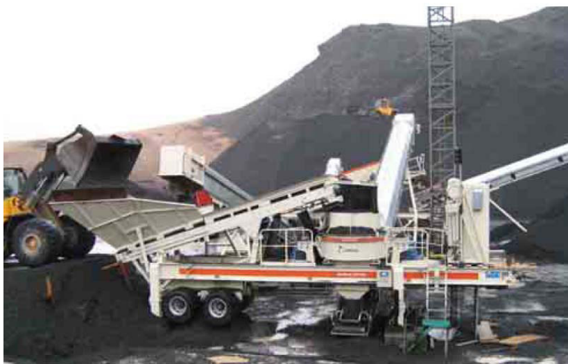
Figure 1: Picture of a typical semi-mobile processing plant to be used at Ironclad's Wilcherry Hill mining operation.
