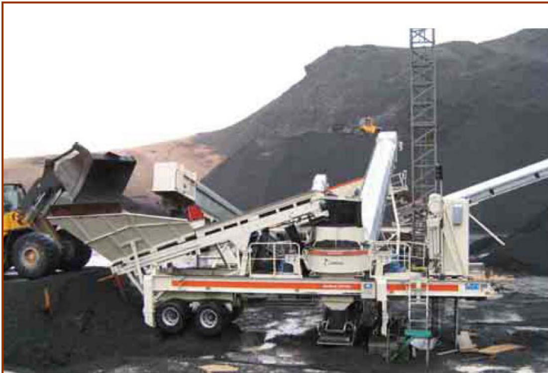
Fig 1 : Proposed Mobile Crushing and Screening Plant (the above is not the property of the Company).
