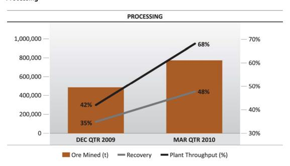
The processing plant continued to perform well, with improving recovery performance and production levels. During the quarter a total of 778,000 tonnes of ore was milled at an average recovery of 48% for the quarter. The recovery performance was improved through the introduction of a new reagent regime, designed to control the altered material present in the ore. Recovery performance improved each month and averaged 52% for March 2010.
