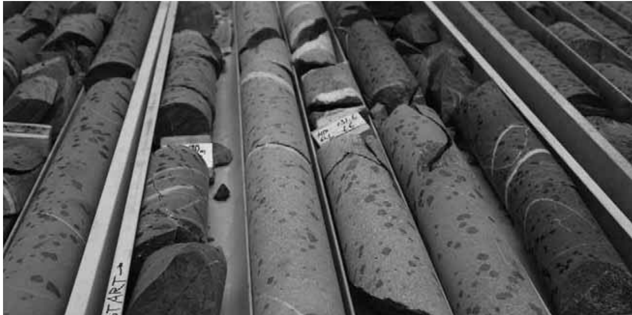
All Nations Drill core with some altered dyke and quartz veins
