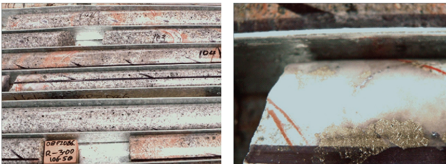
Figure 10: Gromac prospect drill core with zone of intense veining.
