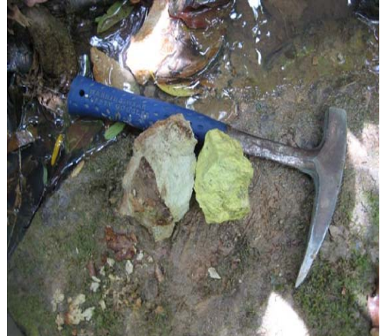
Figure 6: Example of phosphate mineralization within MCPP showing strong reaction with ammonia molybdate (field test for phosphate)
