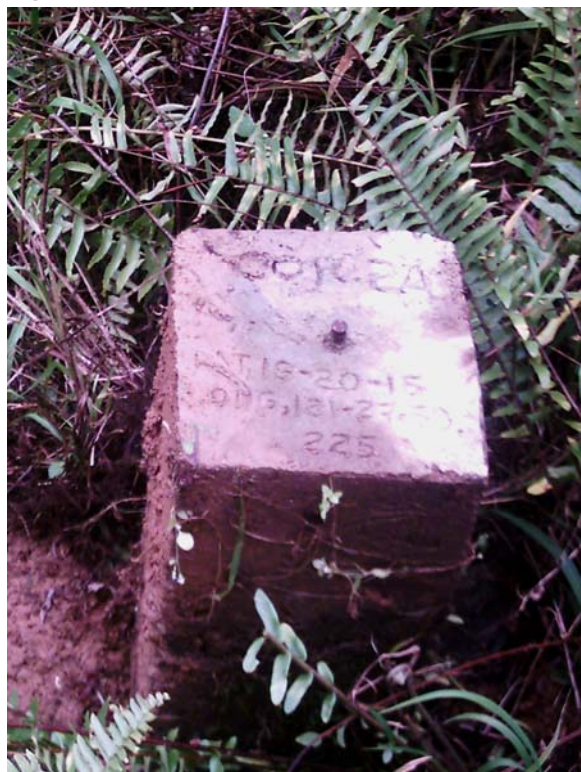
Figure 4-1: NE corner marker for ECC
