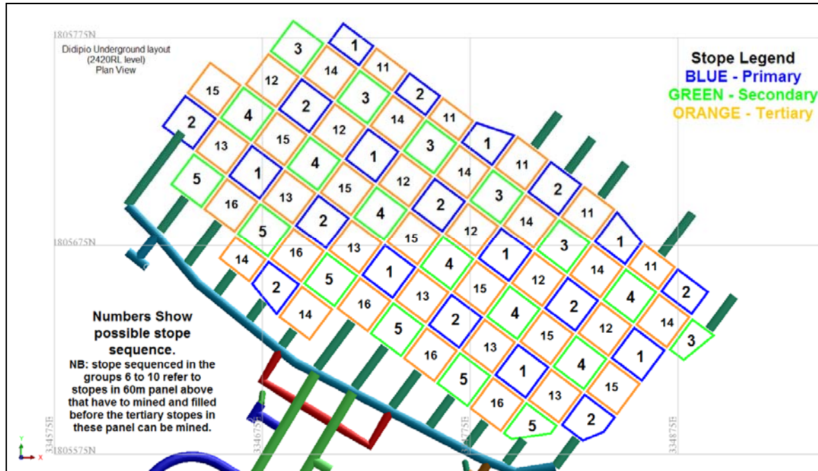
Figure 21-12: Schematic showing stope sequencing
