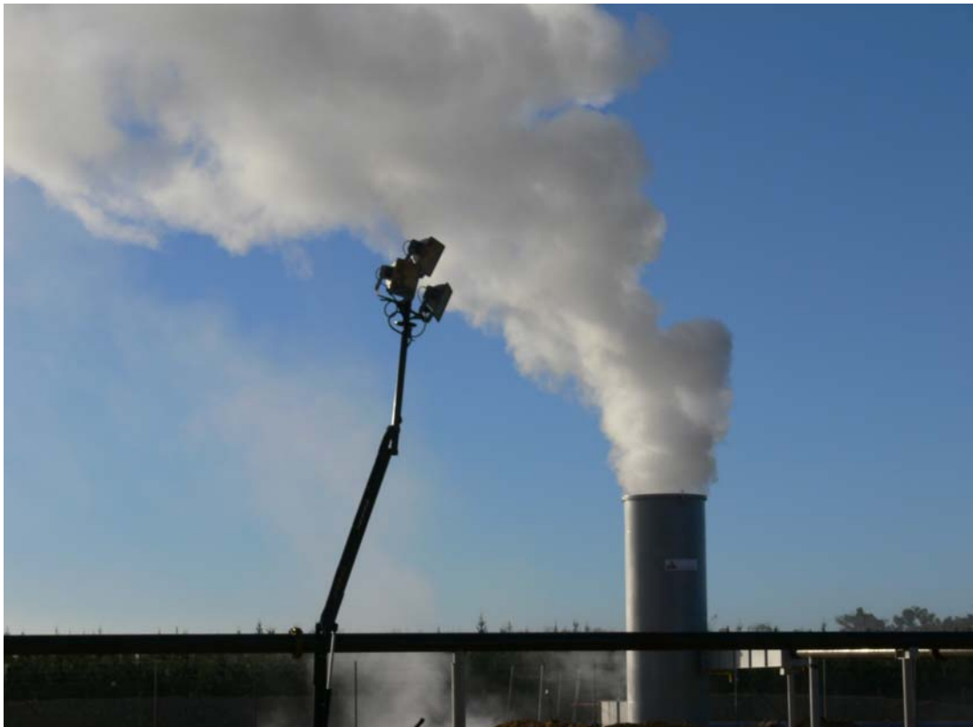
Salamander-1 short flow reservoir test 31 March, 2010; first steam from a hot sedimentary aquifer in Australia.
