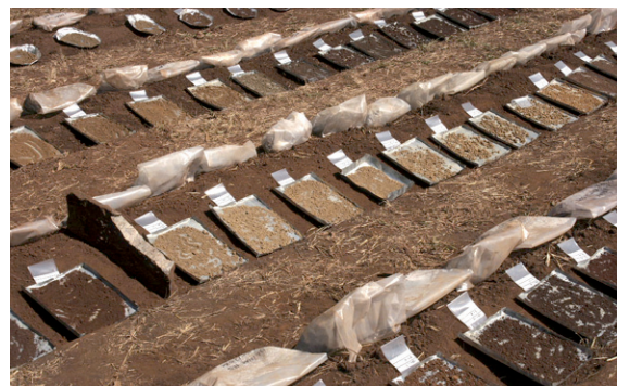
Images: Samples being dried pre XRF analysis.
