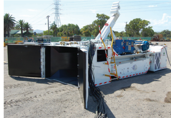
The Guzzler (mobile coal receiving and crushing unit)
