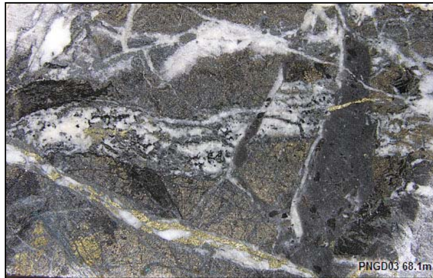
Chalcopyrite and pyrite replacement in brecciated and stockwork fractured intrusive breccia margin. PNGD003 depth 68.1m
