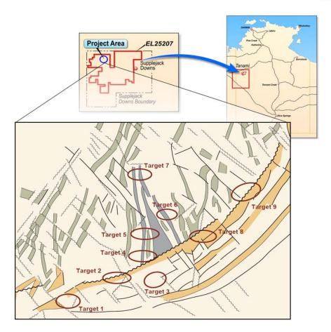
Results from the in-field sampling for non gold mineralization using the x-ray florescence gun and the geological logging will be compiled and assessed. Composite samples to be assayed from targets 4-9 have been sent to the laboratory for assaying.
