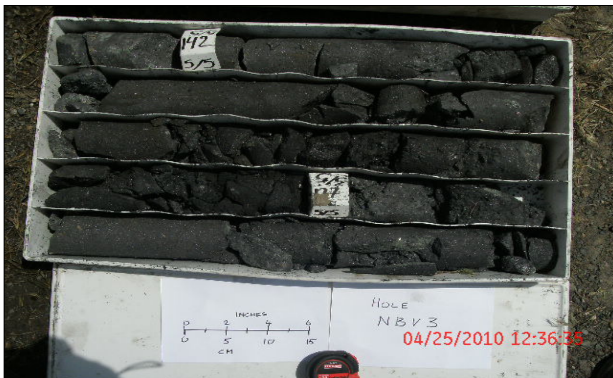
NBV-3 Core: High grade magnetite core from approximately 136' to 142'
