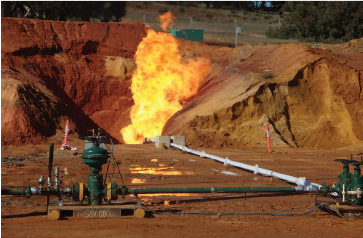
Production testing of Gingin West 1 well on 13 July 2010 (EGO Annual Report 2010, p.17)
