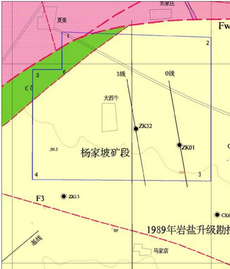
Figure 2. Geology map detail from figure 1 showing permit outline and two drill holes (ZK01 and ZK32) located within the permit.
