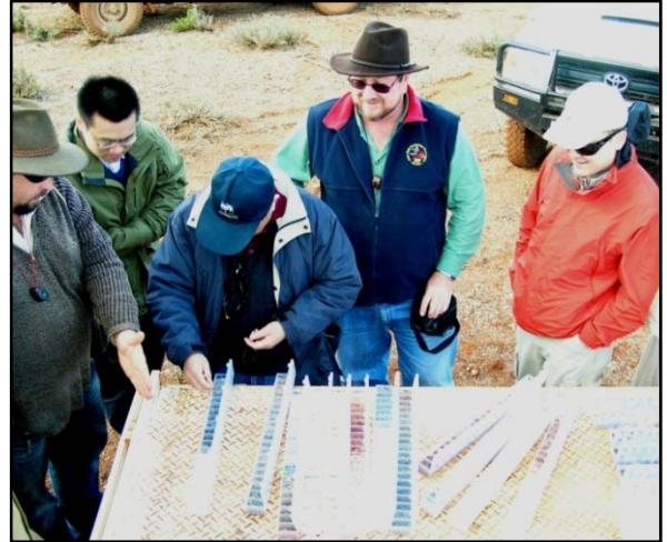
Photo: CITIC representatives examining magnetite and haematite intervals in drill cuttings at Jungle Dam.
