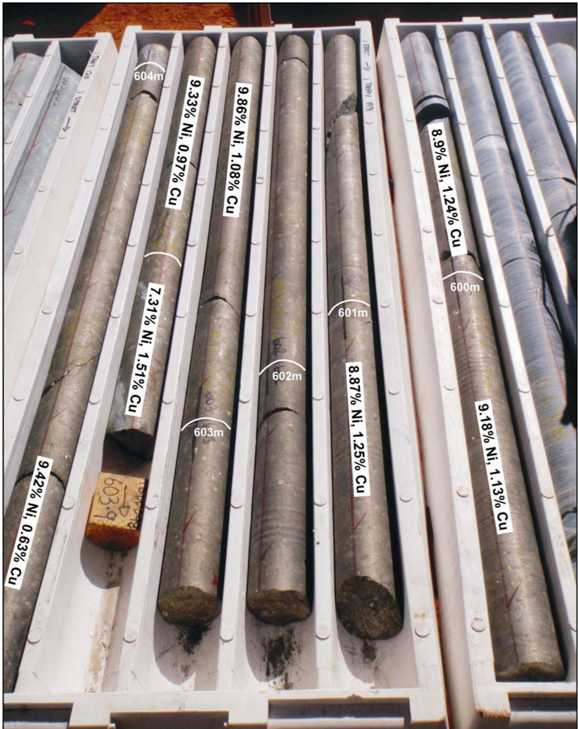
Figure 1: Duketon JV Rosie Prospect - TBDD098 Massive Sulphide Intercept 5.20m @ 9.13% Ni, 1.09% Cu, 0.21% Co and 7.09g/t PGEs (PGEs include 2.22g/t Pt, 1.74g/t Pd, 0.82g/t Rh, 1.79g/t Ru)
