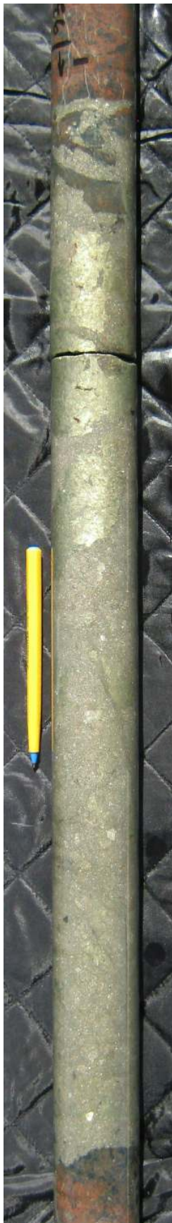
Figure 4: A section of high-grade sulphide-rich drill core (NQ size) from VUD 003
