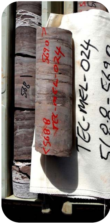
Core sample from Melkor 1 showing horizontally layered siltstone (Billy Creek Formation, 570m).
