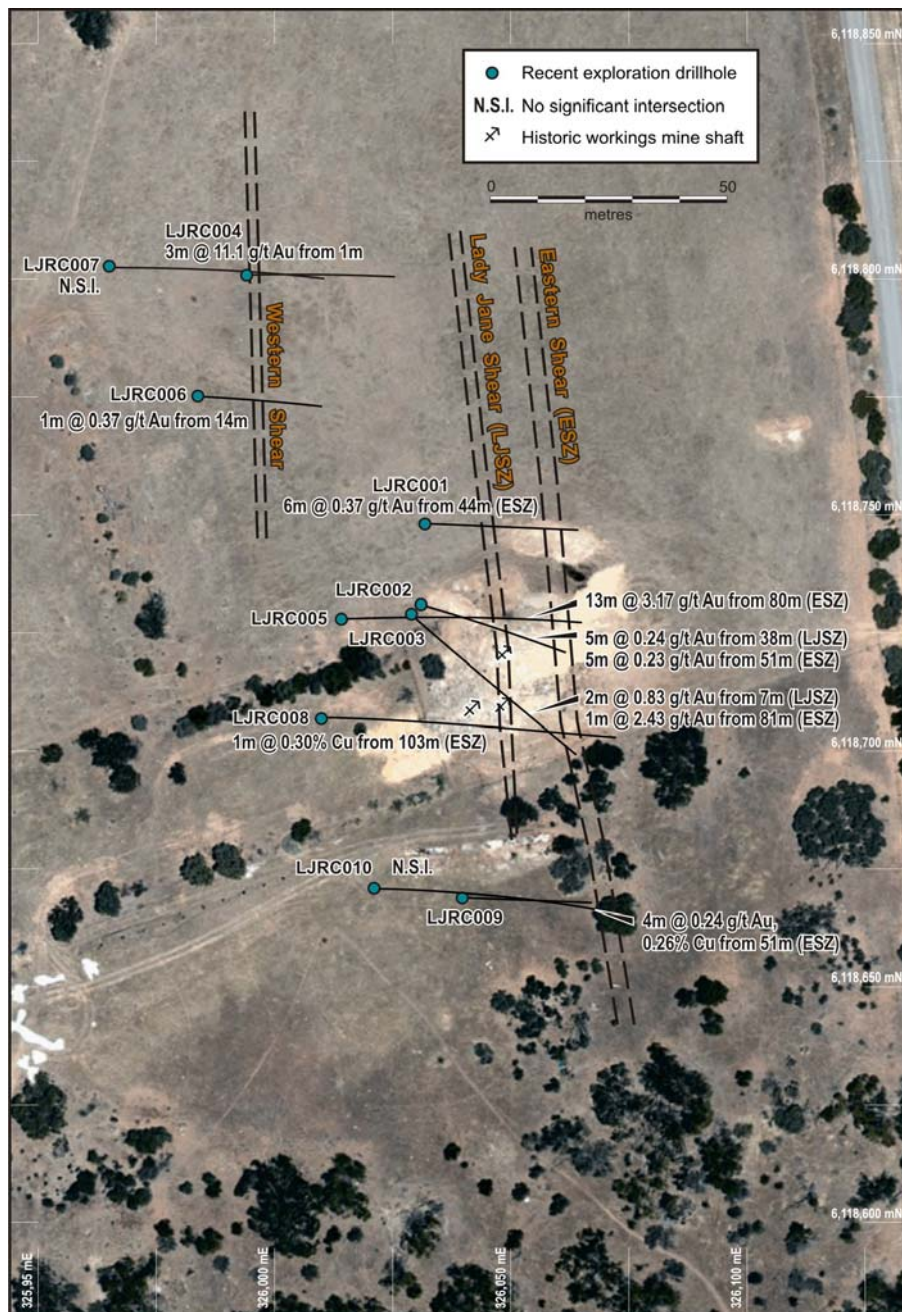
Figure 2. Plan of Lady Jane Prospect area showing recent drilling and anomalous results (Au>0.2 g/t Au and/or Cu>0.25% Cu)
