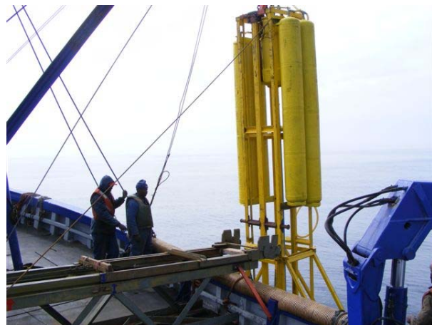
Vibracorer in operation
