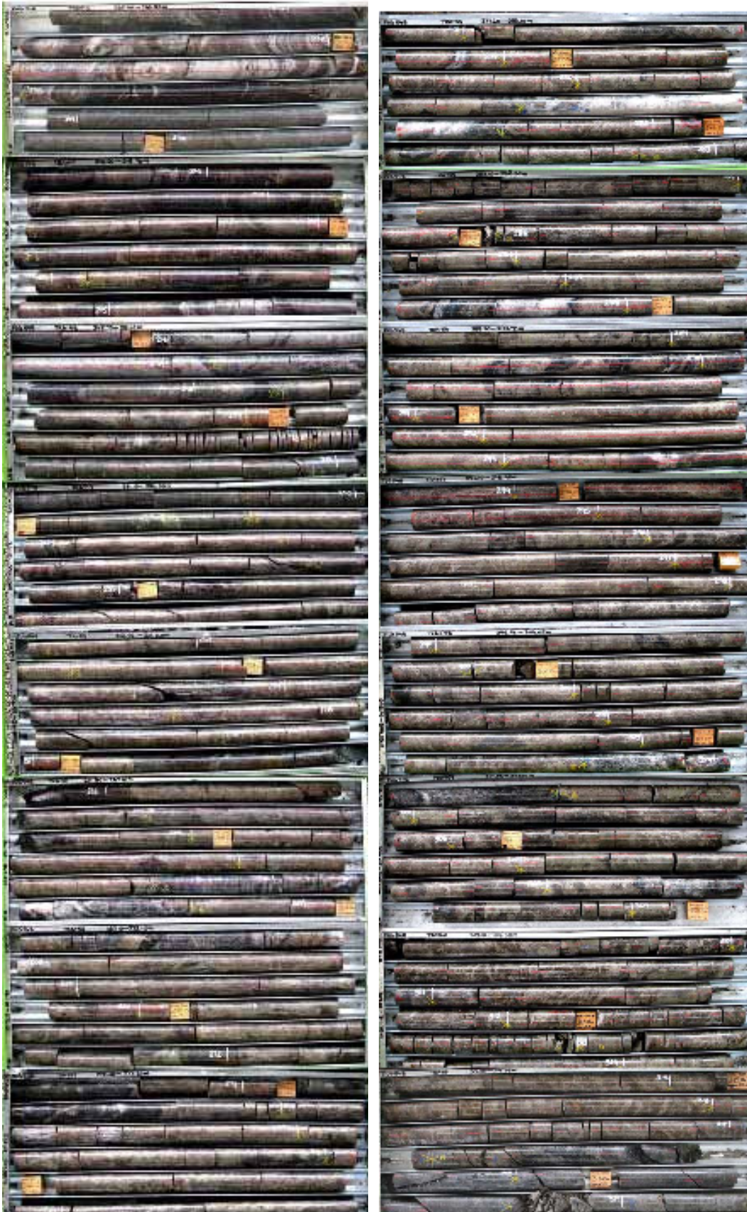
Figure 3: Flying Fox T5 - drill core from FUG 548 which intersected 78.0m @ 9.3% nickel
