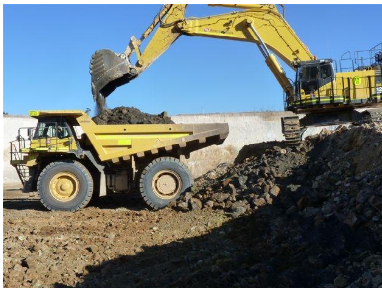
Figure 1: Mining high grade supergene sulphide mineralisation in Tim King Pit
