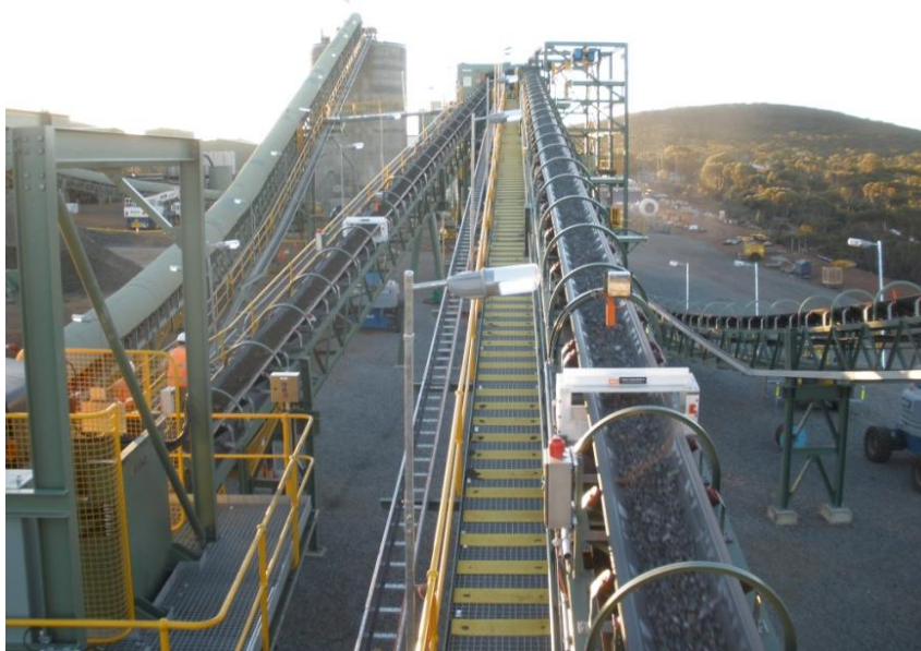
Figure 2: New crushing circuit at Cosmic Boy plant in operation. This has capacity up to 1.0M tpa ore.
