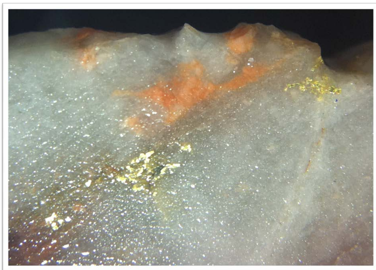
Figure 1. Photograph of Visible Gold in a quartz vein from hole BCRD100002 at Buccaneer. Photo field of view is approximately 3cm across.
