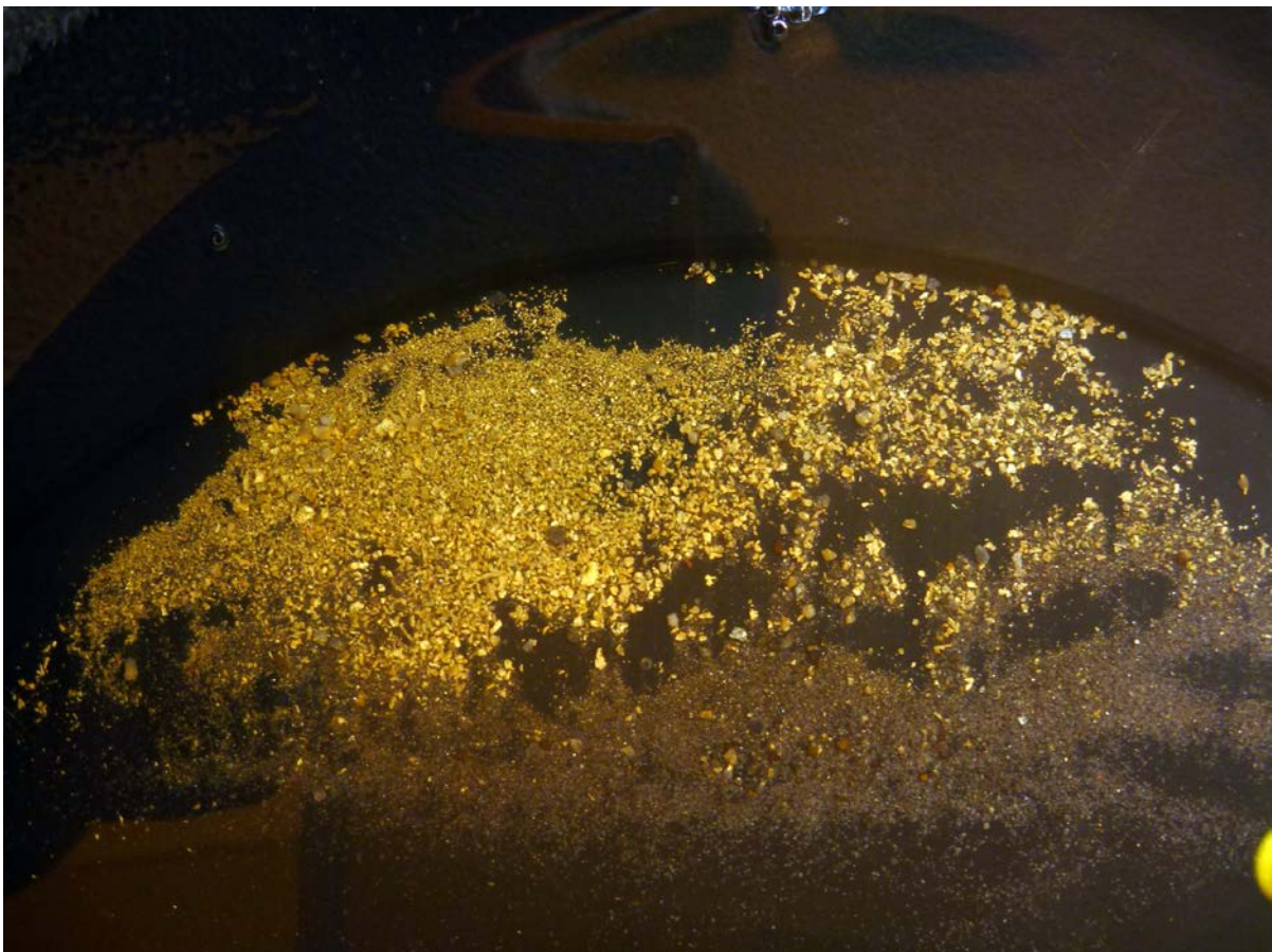
Figure 1. Visible gold grains panned from approximately 4 kilograms of RC drilling sample from 231m to 232m depth in hole OPRC100021. Field of view is approximately 20 centimetres with gold grains up to 5mm. Assays pending.
