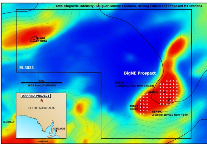
Figure 1: Warrina Project showing proposed MT stations at the BigNE prospect. Background image is Total Magnetic Intensity overlain with Bouger Gravity Contours.
