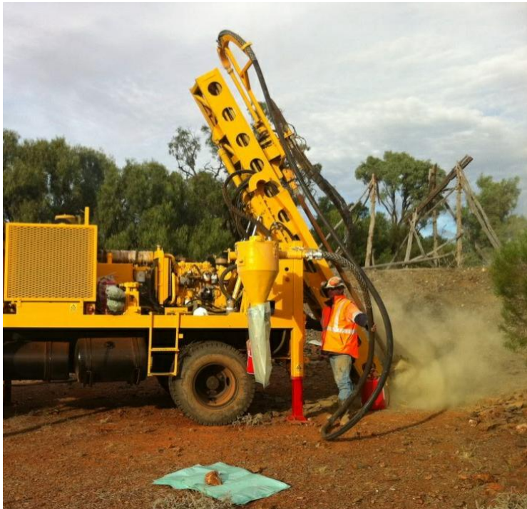
Figure 1 RC drill rig at the Perseverance Mine 22 May 2011
