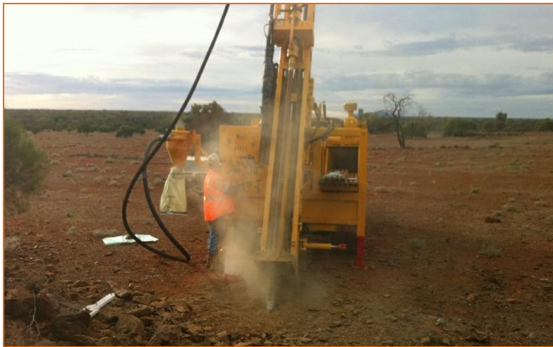
Figure 4 RC Drilling at Perseverance
