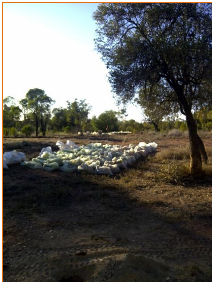
Figure 3 RC samples along strike of Dijoe Gold Mine Shaft
