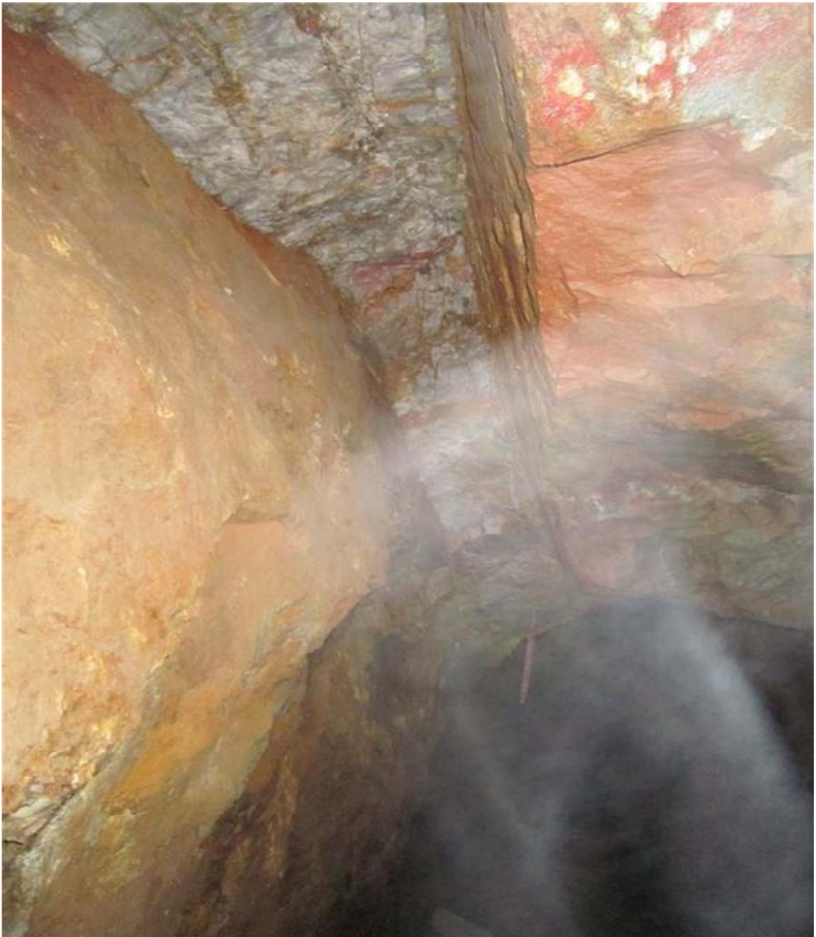
Figure 8 Kargana (Blue Eyes) Gold-hosted Quartz Vein (top-left) on backs of underground drive development. View is approximately 2.5m across
