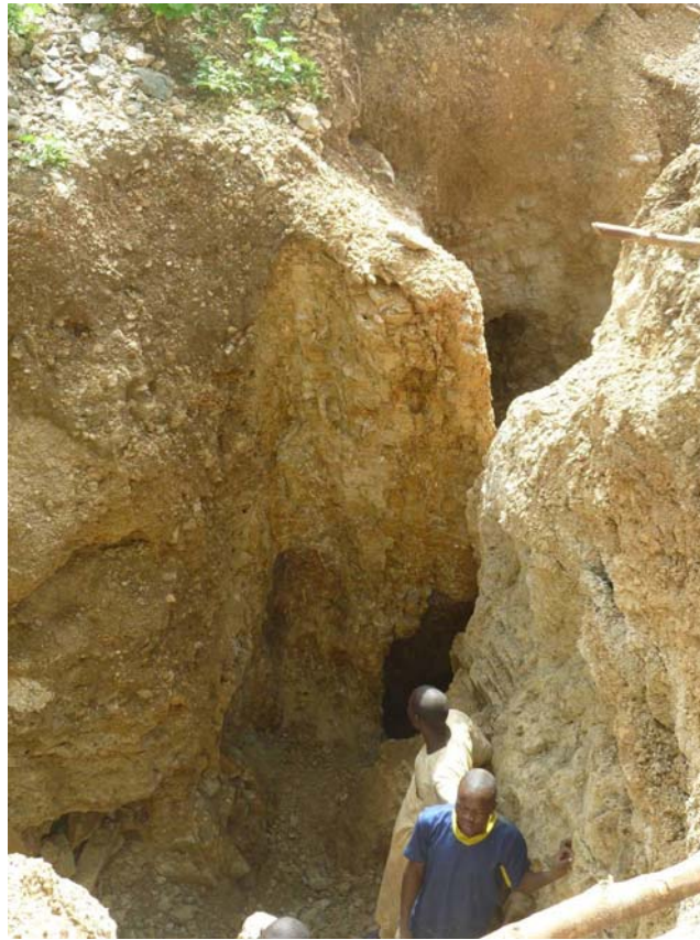
Photo 1 Yargarma workings in intensely sheared and altered rock with quartz veinlets
