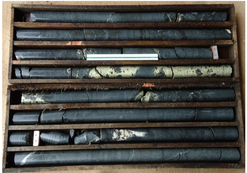
Serra Verde drill hole ASVD-05. Disseminated, stringer and semi-massive chalcopyrite over 13.95m, results pending.
