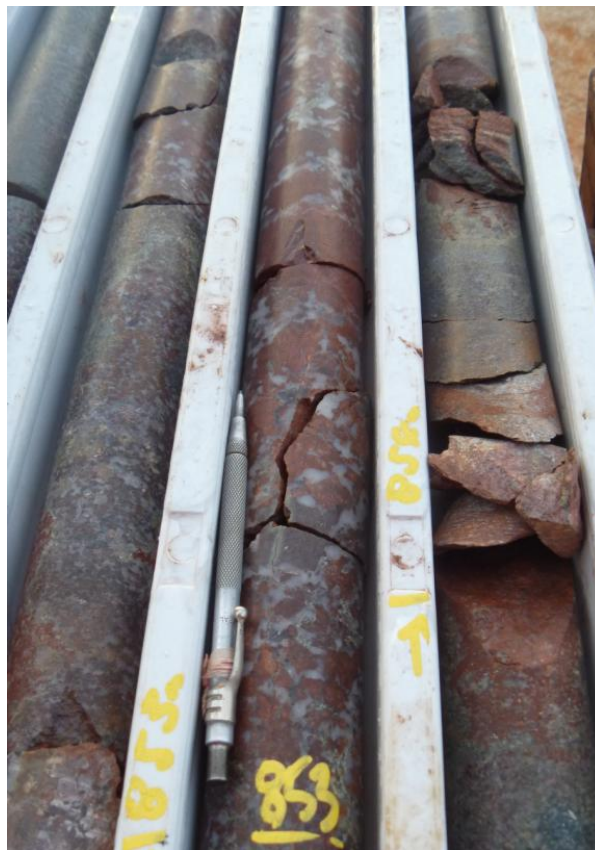
Figure 3: NQ2 core illustrating typical granite pegmatite development in basement intervals of hole ODSDH001.
