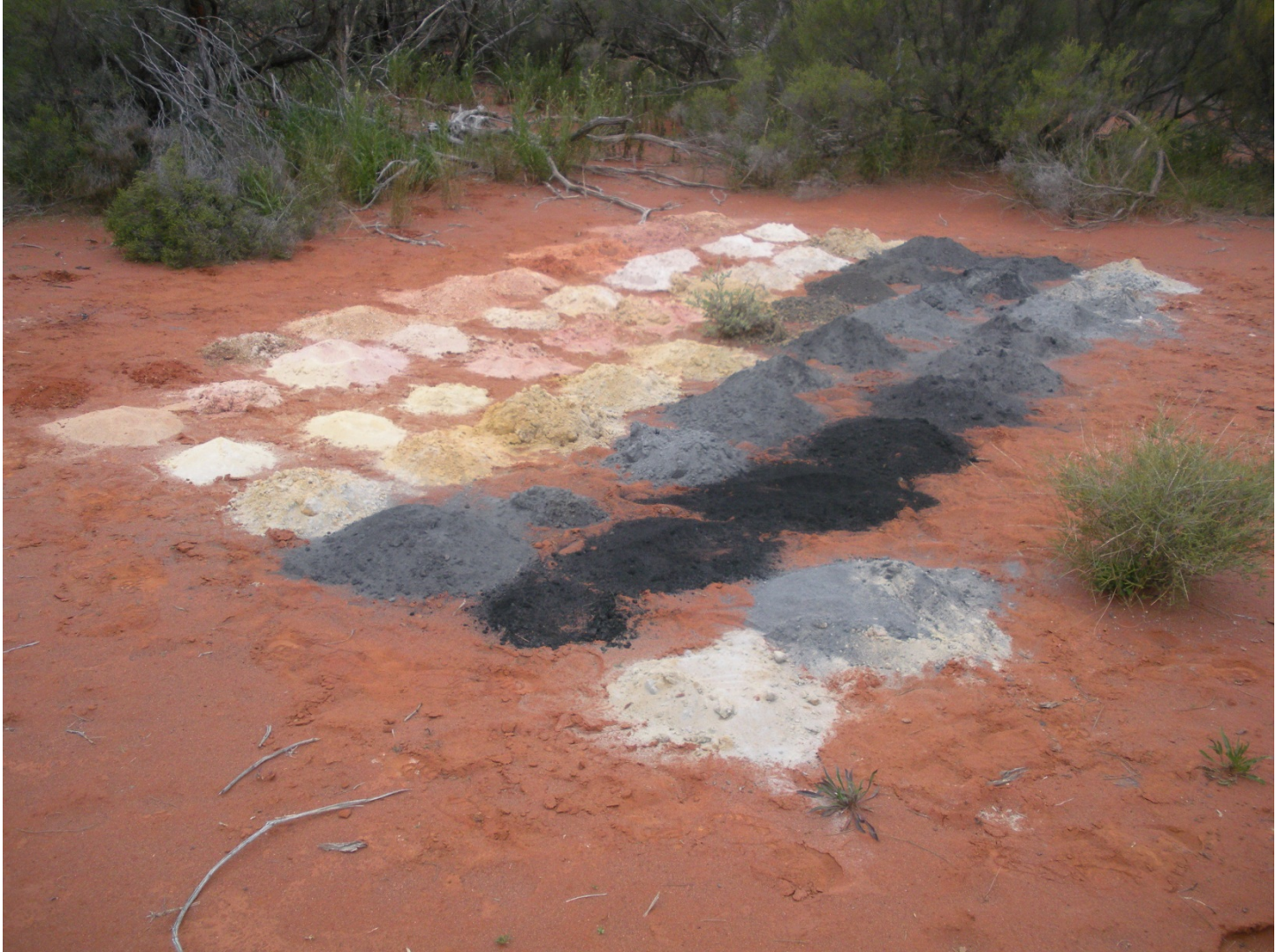
Figure 2 One metre drill chip recovery piles from aircore hole Tal-006 showing the coal seam intercept (in black) from 50m-54m.
