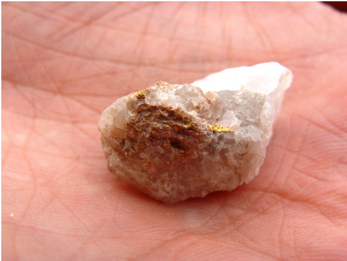
Figure 3 - Visible gold in vein quartz recovered from an in situ quartz vein in the artisanal working located approximately 1000 metres from the Smarts pit.
