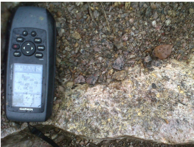
Figure 8 - Yellow secondary uranium mineralisation (believed to be carnotite) developed on fracture plane within radioactively anomalous (~1,000cps) granite (Kaituma anomaly).
