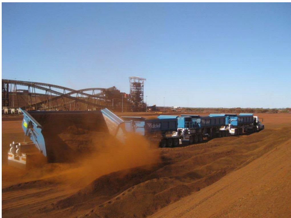
Figure 3: NIOJV Powertrans pit hauler dumping Bonnie Fines at Christmas Creek
