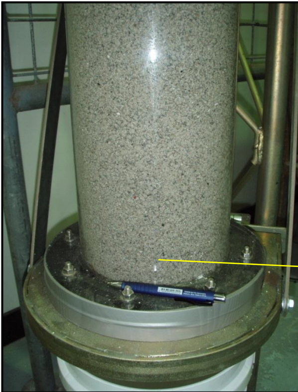
Structure of the ore bed was visually uniform over the full height of the column.
