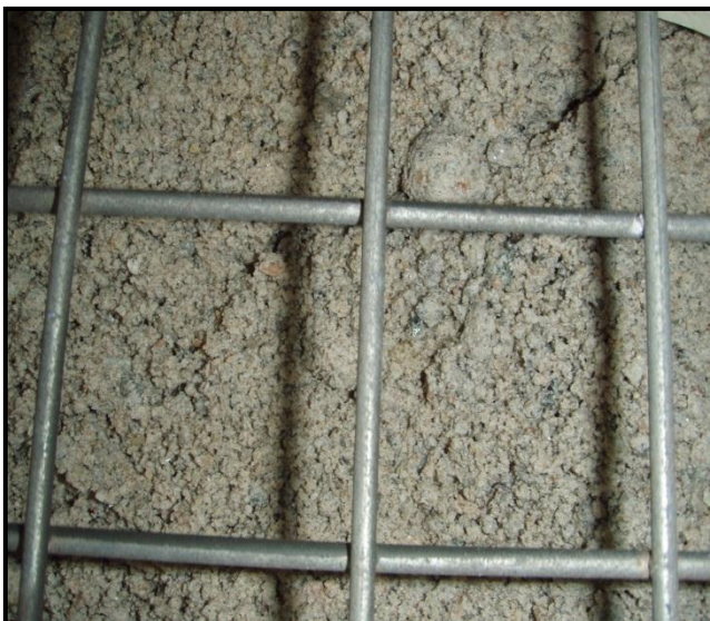
← The top 1m of the column was detached and poured in trays – robust agglomerate structure retained after handling.
