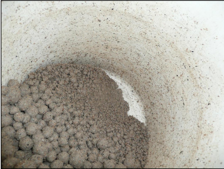
Figure 13-45 Typical Agglomerate 250 g/t MF351 and 6 kg/t Acid Addition
