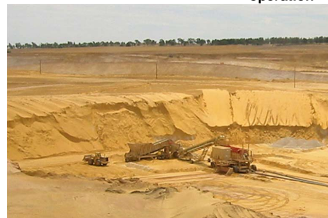
Typical loader and hopper dry mining operation
