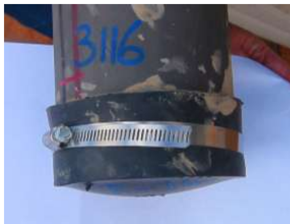
Core sample from Encounter-1 showing rubber end cap bulging due to gas escaping from the shale within the core tube
