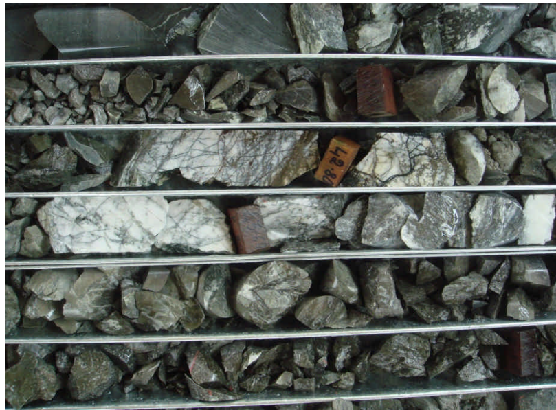
Figure 3: Intersection of quartz veining with sulphide filled fractures returning a grade of 2m at 4.16gpt Au from hole OTMDD002
