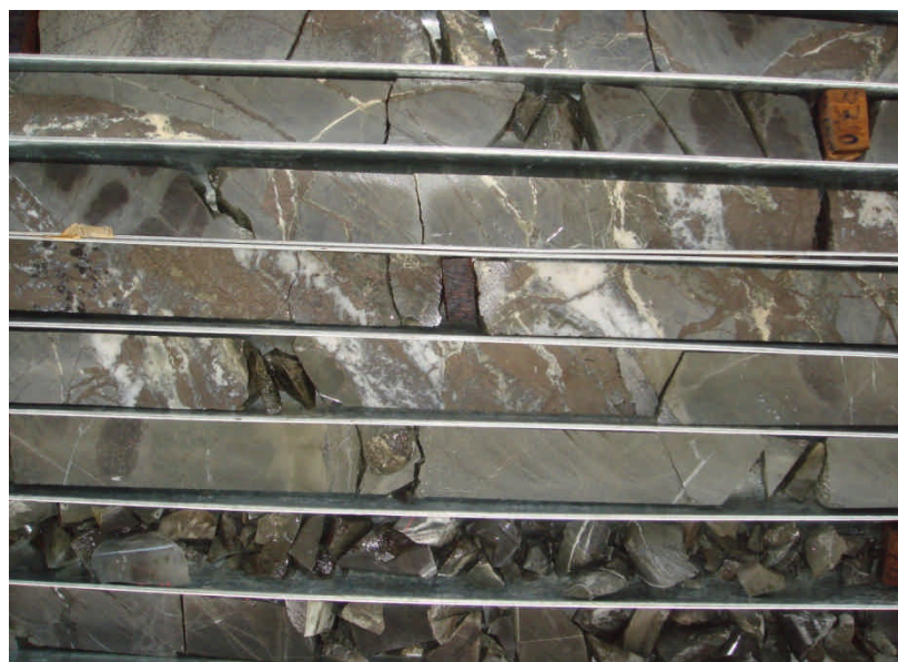
Figure 4: Massive quartz+sulphide veining comprising pyrrhotite+pyrite+chalcopyrite+galena returning an assay of 5.7m @ 5.06gpt Au, including 1m @ 11.1gpt Au from Hole OTSDD002.
